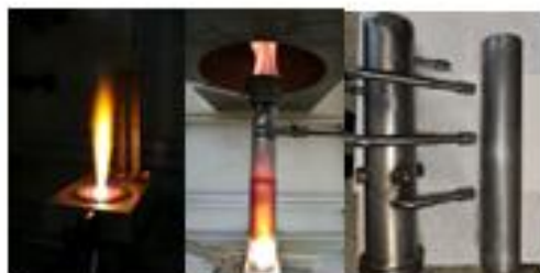
Anoxic FSP Reactor
