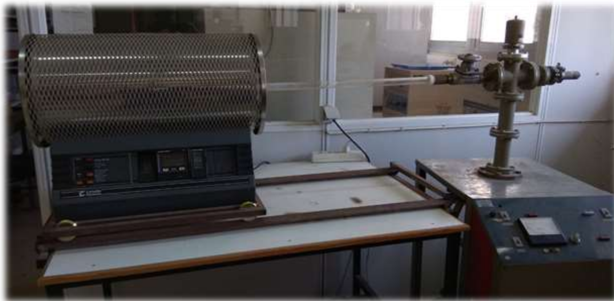
Sample annealing (up to 1000 °C) under continuous vacuum ( 10^{-3} - 10^{-6} Torr )
