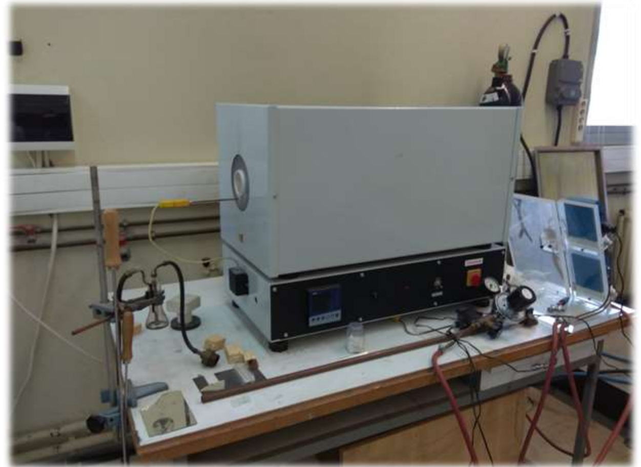
max Temp. 1000 °C with gas flow
