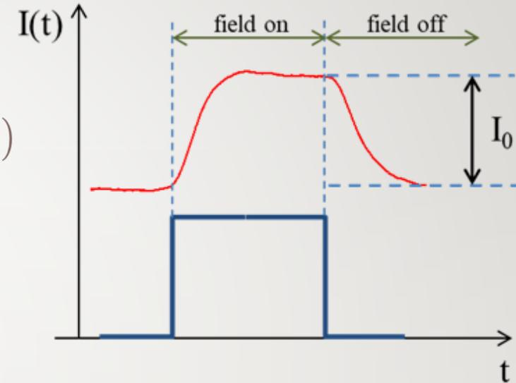
$\Delta n_{max}$ : corresponds to the **steady state birefringence (static birefringence)** when the acoustic field is on
