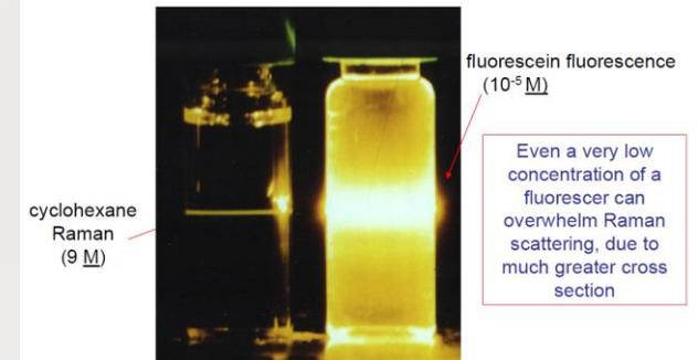
488 nm laser, with 488 rejection filter preceding camera
