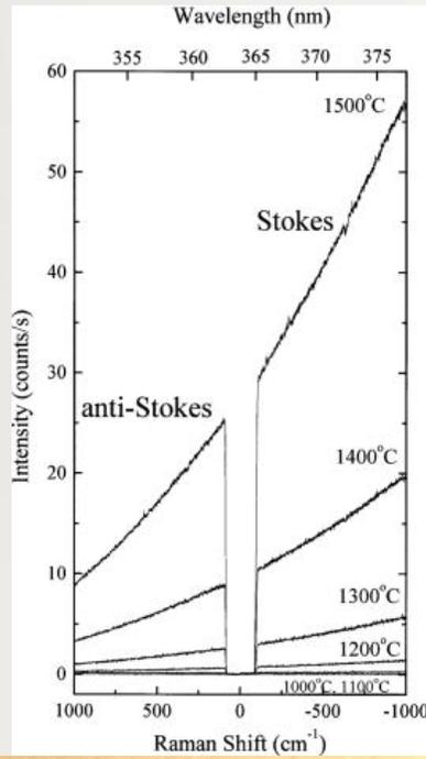
Thermal radiation of furnace and material in the recording range of the Raman spectrum
