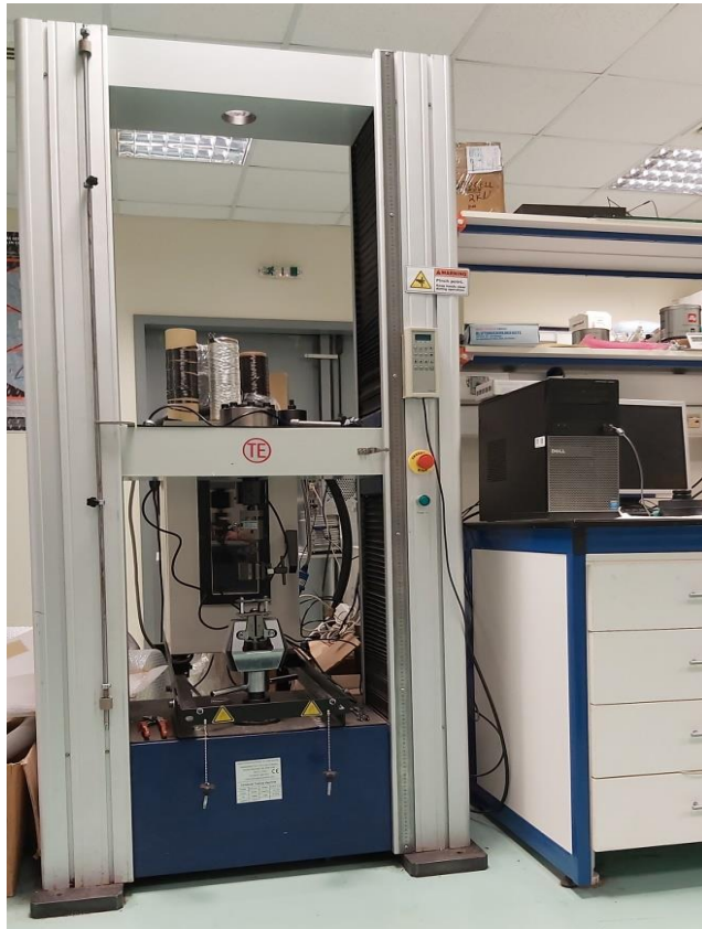
JINAN TESTING EQUIPMENT IE CORPORATION UTS MaxTest software (tensile, compression and bending, 10 kN and 100kN load cell)
