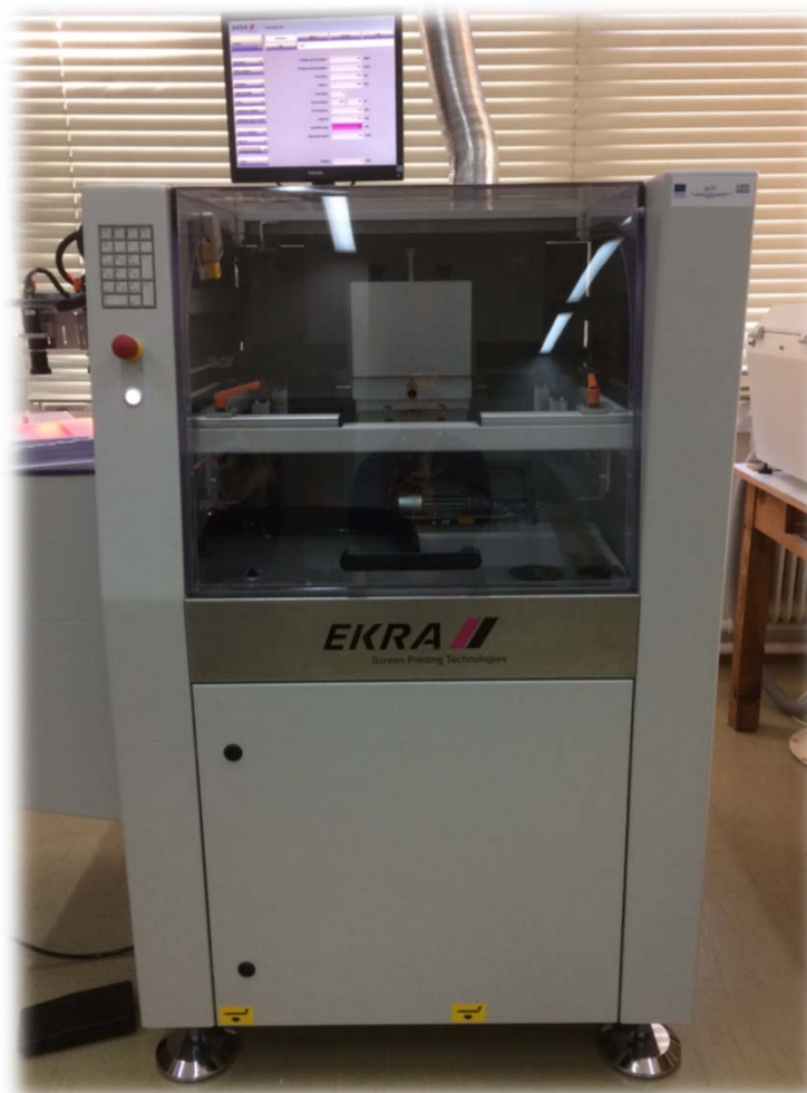
Screen-printer with laser automatic alignment
