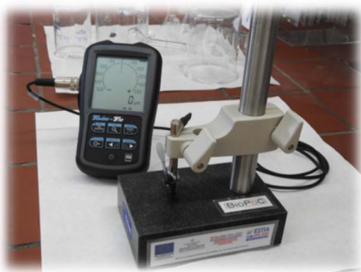
Thickness meter (0.1 \mu\text{m} )
