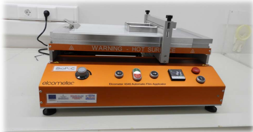
Automatic wet-film applicator (1-50 mil), Temp. 180 °C
