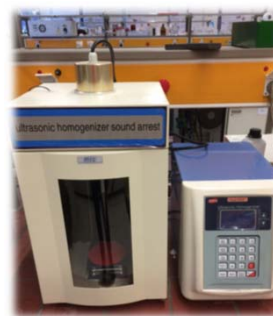
Ultrasonic probe 200 W Exfoliation of layered materials
